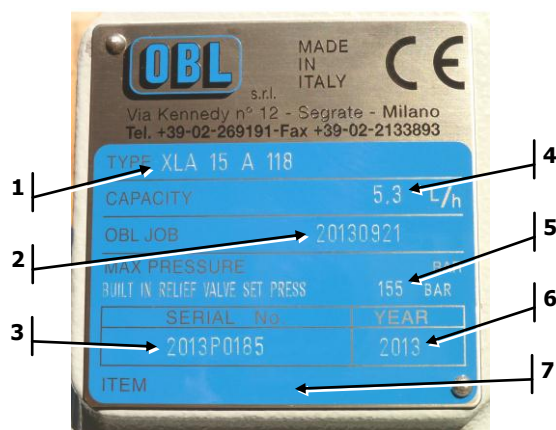
Pump identification nameplate
